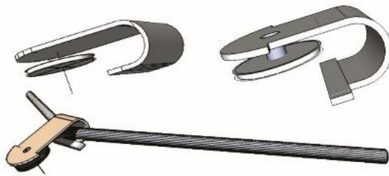
connection of octagonal to bars
