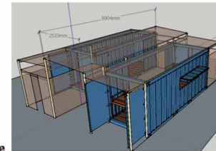
Axo showing Secondary Roof
